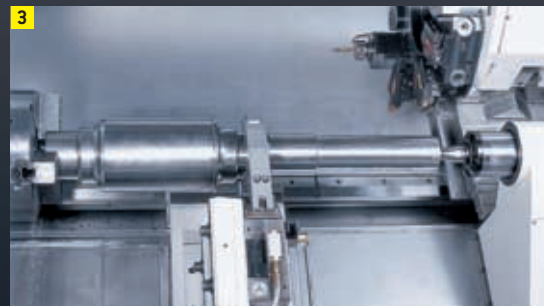
1 Control cabinet with a cable guide 2 Processing with driven tools 3 Shaft parts machining with a tailstock and steady rest
