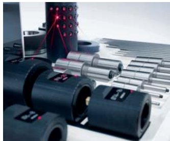
Pick by Light for correct selection of exchange parts
