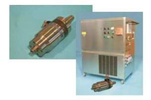
HFK 90 with 380 V AC motor: 42'000 rpm with grease lubrication, 60'000 rpm with oil air lubrication, 2.7 kW, 0.45 Nm, clamping capacity 10 mm, available as turnkey finished system with Supply-Unit 20
