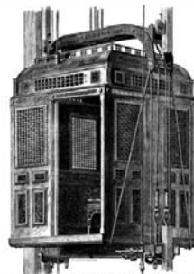
FIG. 1.—THE OTIS ELEVATOR PASSENGER CAR.
