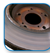
Wear scar in metal showing minor debris deposition on sidewall.
