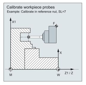
A probe must be calibrated before it can be used. During calibration the triggering points (switching points), positional deviation (skew), and precise ball radius of the workpiece probe are determined and then entered in special data fields \_WP[] in data block GUD6.DEF.
