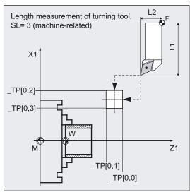
% N T3 MEAS MPF ;Calibration: N10 G0 G18 G94 G90 DIAMOF N20 T7 D1 N30 SUPA Z240 X420 N40 TZL=0.001 PRNUM=1 VMS=0 NMSP=1 N50 MVAR=0 FA=1 TSA=1 MA=2 N60 CYCLE982 N70 GO SUPA Z240 N80 MA=1 N90 CYCLE982 N100 G0 SUPA X350 N110 MA=2 N120 CYCLE982 N130 GO SUPA Z170 N140 MA=1 N150 CYCLE982 N160 G0 SUPA X350 N170 SUPA Z520 N180 SUPA X420 ;Measurement: N200 T3 D1 N210 GO SUPA Z240 X420 N220 MVAR=1 MA=2 TDIF=0.8
