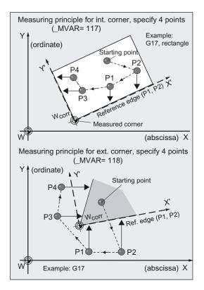
One after the other, points **P2**, P1, P3, P4 are traversed in the cycle with positioning feedrate at positioning height. At each of these points the probe is lowered to measuring depth and then traversed at measuring feedrate parallel to the axis against the workpiece corner.
