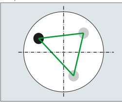
Calibration ball mounted too near the center of rotation; clamped triangle is too small
