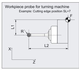
Calibration in a "reference groove" is relative to the machine. In this case, calibration is possible in one cycle call in both axis directions.
