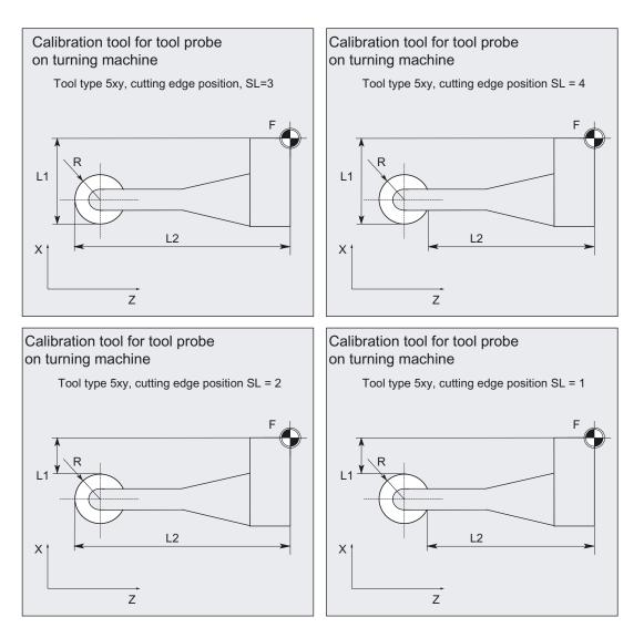
The calibration tool is shaped (bent) in such a way that the probe can be calibrated on all 4 sides with it.
