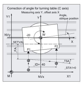
Length 1 (L1) must refer to the center of the probe ball (\_CBIT[14]=0), as for calibration. Careful when positioning! Radius R in length (L1) is ignored.
