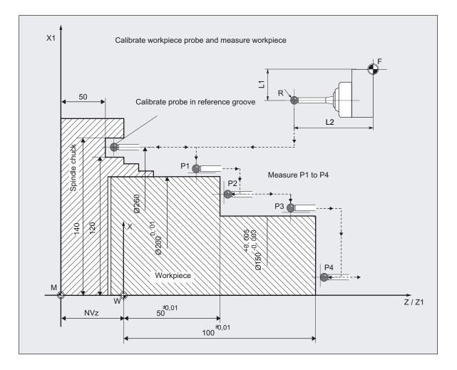
Measuring Cycles for Turning Machines
