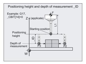
The probe is above the workpiece at positioning height. It must be possible to reach all points without collision.
