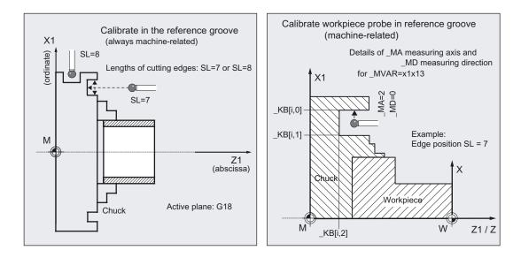
It is also possible to calibrate the position deviation of the probe and the active diameter of the probe ball in both directions.
