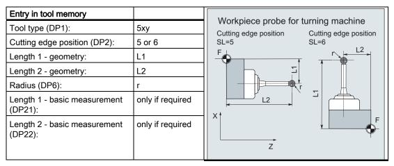
The wear and other tool parameters must be assigned the value 0.
