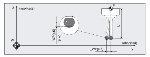
Position deviation and trigger points Tp in X and Y (magnified illustration):
