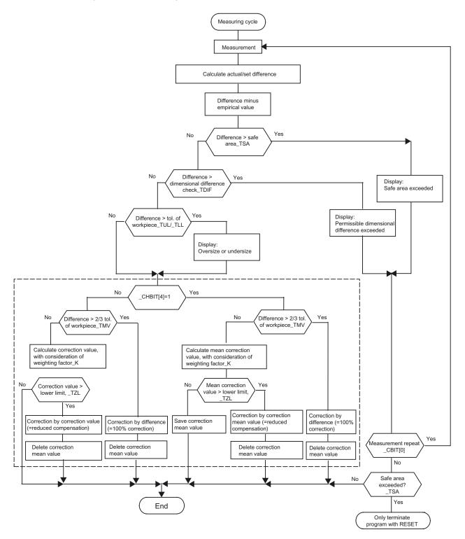
1.12 Overview of measuring cycle functions for milling technology
