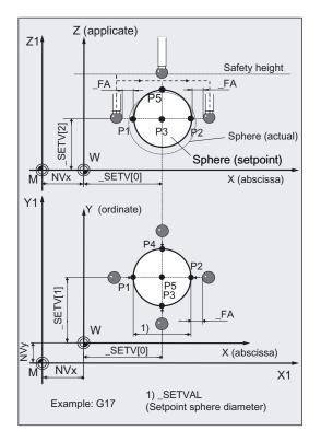
All intermediate positioning actions and measurement movements are paraxial with the active workpiece coordinate system. The measuring points are approached at distance \_FA from the sphere lateral surface (setpoint sphere diameter). Measuring point P1 is approached first. After positioning in the abscissa, ordinate, the applicate is lowered to the
