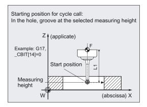
In all measuring variants the probe must be positioned at the required **measuring height** in the applicate (tool axis) close to the first measuring point P1.
