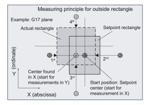
The rectangle lies parallel to the axes of the workpiece coordinate system.
