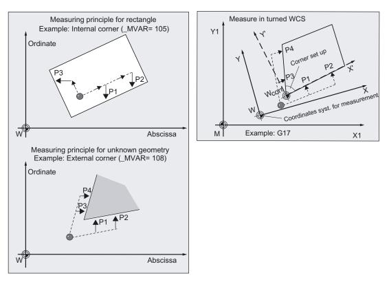
The cycle approaches either 3 (for a rectangle) or 4 measuring points (if workpiece geometry is not known) and calculates the point of intersection of the resulting straight lines and the angle of rotation to the positive abscissa axis of the current plane. If the workpiece geometry is known (rectangle), the corner to be calculated can be offset.
