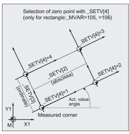
With measuring variants MVAR=105, =106 (rectangle) the measured corner can be selected offset as workpiece zero.
