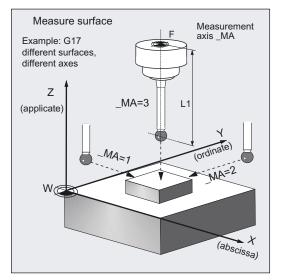
A special measuring variant permits **differential measurement** with the axes of the plane. The special procedure for this measurement permits use of an **uncalibrated** multidirectional probe.
