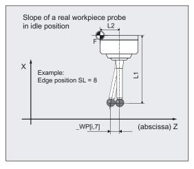
6.4 CYCLE973 Calibrating workpiece probes
