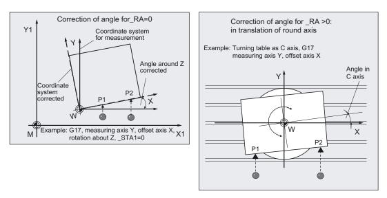
This can be used to determine and correct the rotation component in the zero offset (ZO, frame) of the workpiece in the plane.
