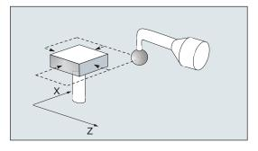
A probe must be calibrated before it can be used. Calibration involves precisely determining the triggering points (switching points) of the tool probe and entering them in special data fields.
