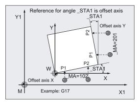
The set angle \_STA1 specifies the required angle between the edge and the positive direction of the offset axis. In the case of \_STA1=0, the edge is aligned paraxially with regards to the offset axis after correction.
