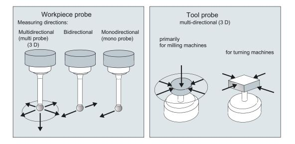
The probe type is defined by a parameter (\_PRNUM) in measuring cycles (see Section 2.10).
