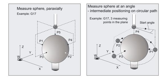
Measurements can be performed **paraxially** with the workpiece coordinates system (WCS) **or at an angle** in the plane.
