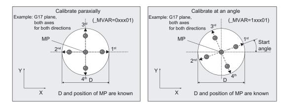
The center point (CP) of the hole and its diameter (D) must be known for this calibration variant!
