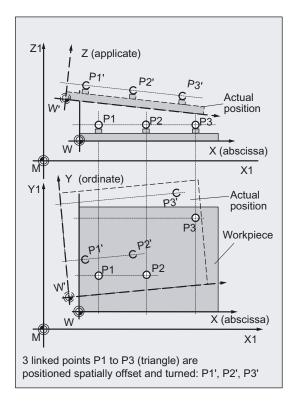
CYCLE119 is called as a subroutine by measuring cycle CYCLE997. To allow this cycle to be used universally, its data are transferred via parameters.
