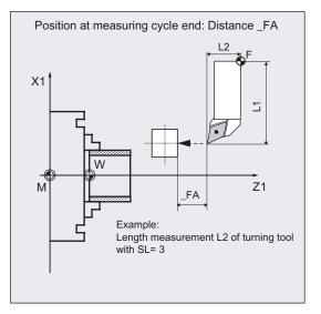
6.3 CYCLE982 tool: Measure turning and milling tools
