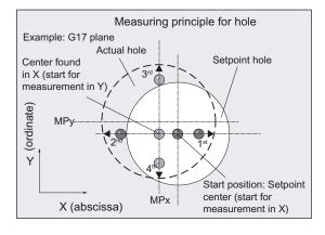
Two points each are measured in the abscissa and ordinate. The actual position of the center point (CP) in relation to workpiece zero is calculated from these four measured values. The actual diameter is calculated from the two points in the ordinate.
