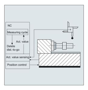
The principle of "on-the-fly" measurement is implemented in the SINUMERIK control. The probe signal is processed directly on the NC so that the delay when acquiring measured values is minimal. This permits a higher measuring speed for the prescribed measuring precision and time needed for measuring is reduced.
