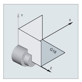
Turning machines generally only use axes Z and X and therefore:
