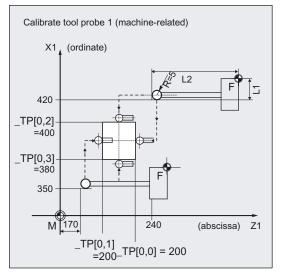
The default values of probe 1 as applied in data block GUD6 with a tolerance of approx. 1 mm:
