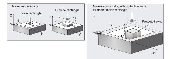
Measurement is performed paraxially to the workpiece coordinate system.
