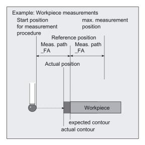
Measurement path \_FA defines the distance between the **starting position** and the expected switching position (**setpoint**) of the probe. \_FA is data type REAL with values >0.
