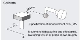
Calibrate in increments as preparation for incremental measurement
