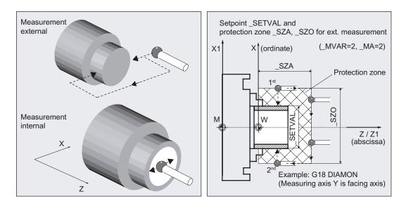
Two opposite measuring points in measuring axis \_MA are approached symmetrically to the workpiece zero at the distance of the setpoint \_SETVAL.
