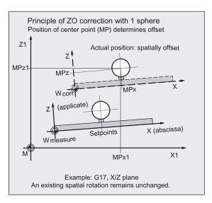
The actual value/setpoint differences of the center point coordinates are included the calculation of the translatory component of the ZO. The offset acts such that the calculated sphere center point in the offset ZO includes the specified setpoint position (workpiece coordinates, three axes).
