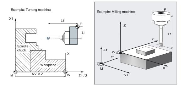
The position of tool reference point F in the machine coordinate system is displayed with machine zero M as the **machine actual value**.
