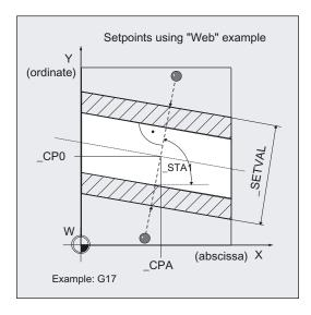
The setpoint for diameter or width is specified in \_SETVAL.
