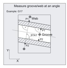
The actual value of the groove width and web width and the position of the groove center and web center in relation to workpiece zero are calculated from the measured values.
