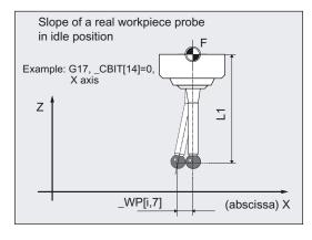
A real workpiece probe can deviate from its ideal vertical position even when not deflected. This positional deviation (skew) can be determined with measuring variants in this cycle and then entered in the intended array of the workpiece \_WP[i, 7] for abscissa and \_WP[i, 8] for ordinate (for detailed data: refer to Data description chapter "Cycle data").
