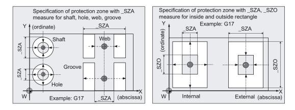
The safety zone (diameter or width) for shaft, hole, web, and groove is defined in \_SZA.
