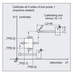
To obtain a minimum measurement path of 1 mm, the measurement path is programmed with  $_FA = 1+5= 6$  mm (max. total measurement path = 12 mm).
