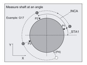
The position of the points is determined by starting angle \_STA1, indexing angles \_INCA, the diameter and the set center point.
