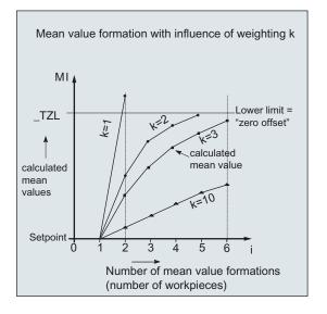
Computational characteristic of the mean value with different weightings k
