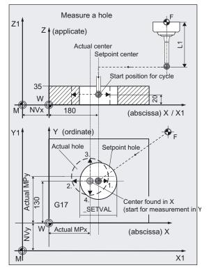
The hole was machined with milling tool **T20**, **D1** in the same environment as for measuring (G17, ...) with circular milling.
