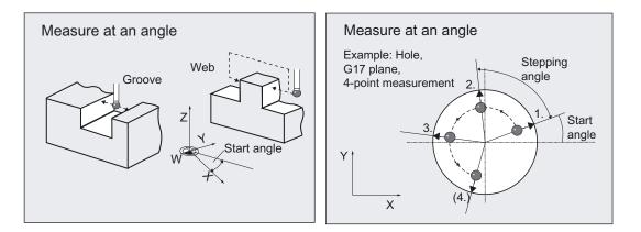
Measurement is performed at a specified starting angle to the abscissa of the workpiece coordinate system.
