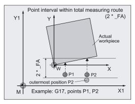
The position of the corner is selected with all 4 points. So for a rectangle, for example, different corners can be selected as the zero point depending on whether measuring variant internal or external corner is applied.
