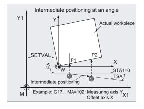
The probe is positioned with respect to the surface to be measured in such a way that during traversal of the measuring axis <u>MA</u> specified in the direction of the setpoint **\_SETVALmeasuring point 1** on the surface will be reached.
