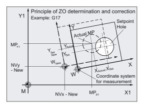
The angular position cannot be determined with this cycle.
