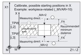
Transformations can be activated in workpiece-related measurement, calibration.
