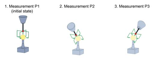
With the 2nd and 3rd measurements, the rotary axis to be measured is rotated around the largest possible angle. The position of the calibration ball must be stationary during measurement (1st, 2nd, 3rd).
