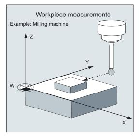
In workpiece measurement, a measuring probe is moved up to the clamped workpiece in the same way as a tool and the measured values are acquired. The flexibility of measuring cycles makes it possible to perform nearly all measurements required on a milling or turning machine.
