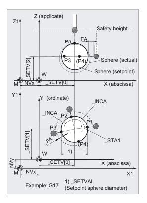
With \_STA1 (starting angle) the angle position of P1 is defined, with \_INCA, the incremental angle after P2 and then after P3. If the measuring variant is selected with 4 measuring points on a circle (\_MVAR=1x1109), \_INCA is also valid from P3 to P4.
