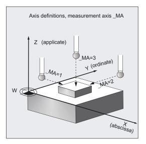
With some measuring variants, for example, in CYCLE998, positioning in another axis that must be defined, also called offset axis can be performed between measurements in the measuring axis. This must be defined in parameter \_MA with offset axis/measuring axis. The higher digit codes the offset axis, the lower digit the measuring axis, the tens digit is 0.
