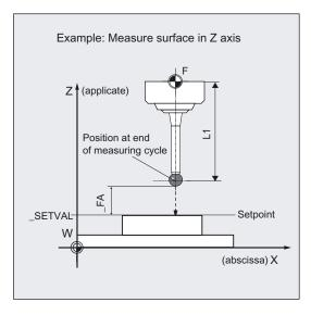
The absolute value of the positional deviation from the setpoint must not be greater than the measuring path \_FA. Otherwise, no measurement will be performed.
