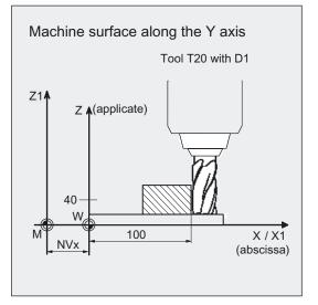
This tool offset will therefore affect the production of the next workpieces or possible remachining.
