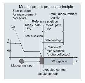
The procedure is described using the **workpiece measurement**. The procedure is the same for tool measurement. In this case, however, the tool is moved and the probe is fixed.
