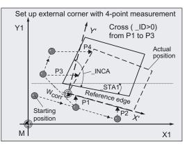
Length 1 (L1) must refer to the center of the probe ball (\_CBIT[14]=0), as for calibration. Careful when positioning! Radius R in length (L1) is ignored.
