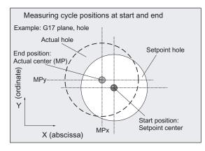
When measurement is complete the probe is positioned above the **calculated** center point or center at starting position height.
