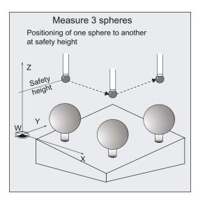
The cycle starts with measurement of the 1st sphere. Active G17 to G19 defines the plane with abscissa, ordinate. The applicate is the infeed axis.
