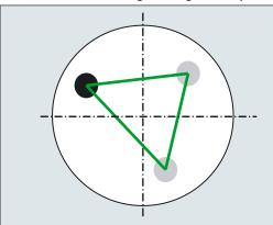
Rotary axis positions poorly selected; clamped triangle is too small
