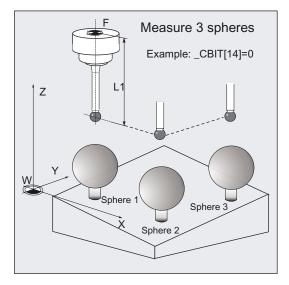
Measurement is performed in all three coordinate axes.
