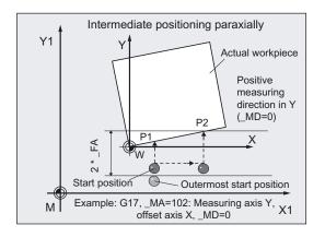
The probe is positioned with respect to the surface to be measured in such a way that during traversal in the specified measuring axis \_MA and direction of the measurement in \_MD both measuring points on the surface within the total measurement path:  $2 \cdot _FA$  in mm is reached.
