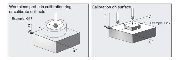
The probe trigger points must be determined in the axis directions that are dependent on:
