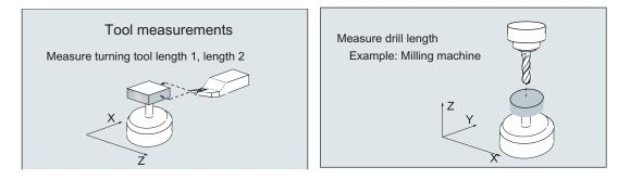
In tool measurement, the selected tool is moved up to the probe and the measured values are acquired. The probe is either in a fixed in position or is swung into the working area with a mechanism. The tool geometry measured is entered in the appropriate tool offset data set.
