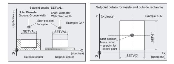
The position of the probe in the abscissa, ordinate at the beginning of a cycle is evaluated for the setpoint of the center point of a hole, shaft, or rectangle, or for the center of a groove, web.
