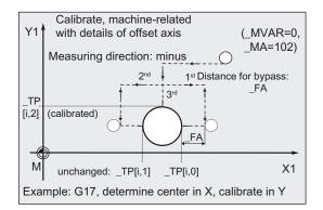
Additionally specifying the offset axis in \_MA (\_MA= 102 or \_MA= 201) first causes the exact center of the tool probe to be detected in the offset axis before calibration takes place in the measuring axis.
