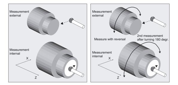
The measuring cycle determines the actual value of the workpiece with respect to the workpiece zero in the selected measuring axis \_MA and calculates the difference from a defined setpoint (setpoint-actual value).
