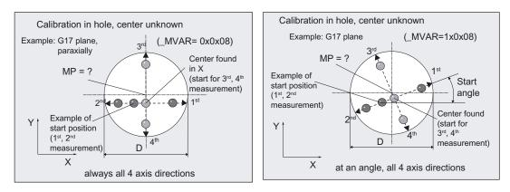
In this measuring variant first the hole center and then the positional deviation (skew) of the probe is calculated. Then the trigger points in all 4 axis directions on the plane are calculated.
