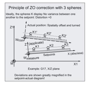
Compensation of the entire active frame with its translational and rotary components is performed after 3 spheres have been measured with cycle CYCLE119 (see following section).
