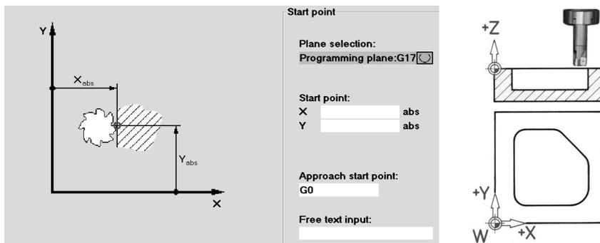
If the shown coordinate system is turned correspondingly, the axes and their directions in the associated working plane will change (DIN 66217).
