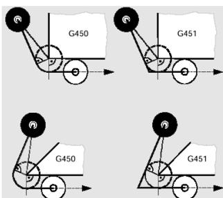
\* A tangential approach of the point via an intermediate point at X5/Y6-12 (with G41 active) would be better in view of the manufacturing technology. The procedure selected here (angle between approaching path and first contour straight line < 180°, i.e. starting point before the contour) is normally easier as regards the program: If the first contour element is not paraxial, the exact intermediate point must be calculated.
