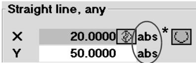
By using the softkey **Alternative**, you can switch over at any time.
