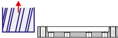
With rapid traverse (G0), the cutter is traversed away from the workpiece in Z direction. At the same time, the spindle is stopped with M5 and the coolant is turned off with M9.
