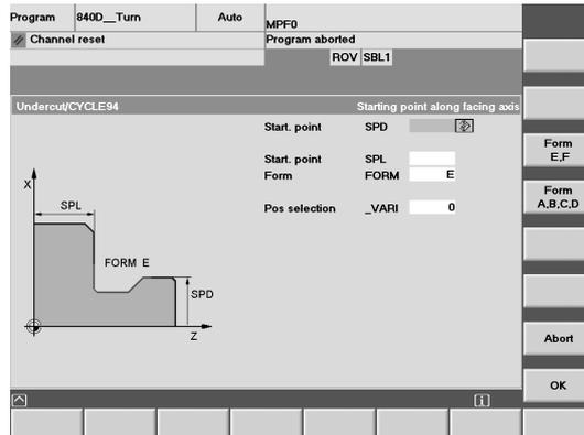
Select the appropriate softkeys to call the input window for the undercut cycle.
