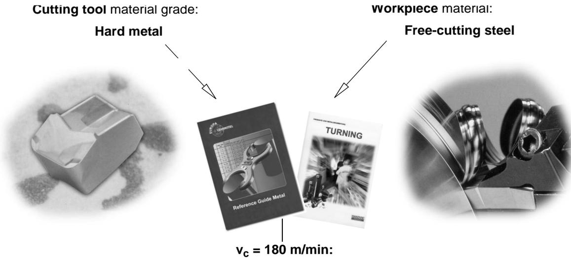
**Constant cutting rate  $v_c$  (G96) when roughing, finishing and plunge-cutting:**
