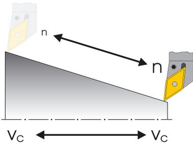
To make sure that the selected cutting rate is observed on each workpiece diameter, the appropriate speed is adapted by the control system using the command G96 = constant cutting rate. This is carried out using either d.c. motors or variable-frequency three-phase motors.
