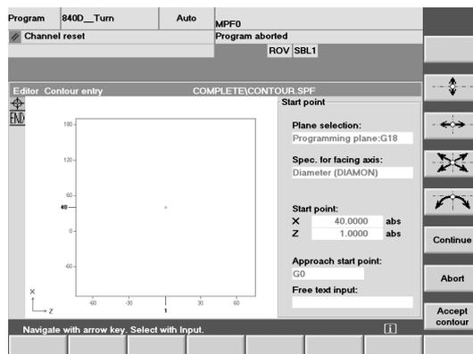
Instead of thinking in cryptic G commands, you can also create the contour definition using simple pictographs (see vertical softkey bar).
