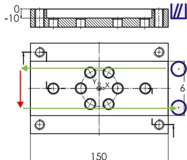
In this first example, the contour is finished without taking into account the cutter radius automatically, i.e. the center point path of the cutter is programmed:
