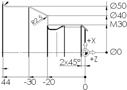
Approaching the contour of X24/Z1 and the machining of the 45° chamfer can be done in one block.
