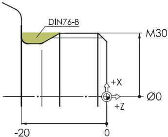
A position is approached at rapid traverse from which the starting position of the undercut can be reached without crash.
