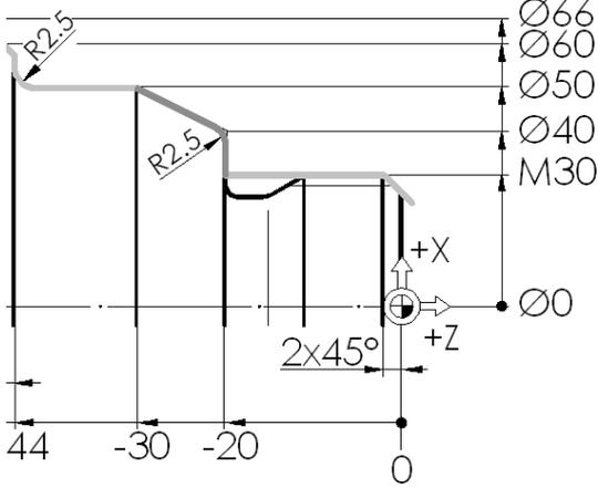
Vertical on X40. The transition to the oblique line at X50/Z-30 will be rounded with 2.5 mm (RND = Rounding).
