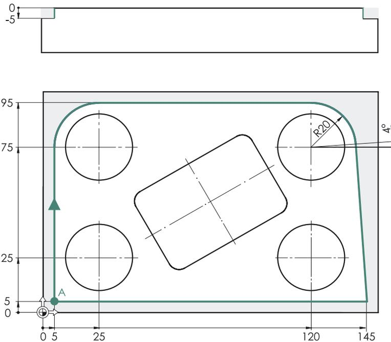
The material is to be shaped by cutting along the contour marked in blue by means of a 20mm end mill.
