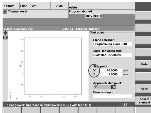
The contour definition starts 1 mm in X and 1 mm in Z before the first contour point.
