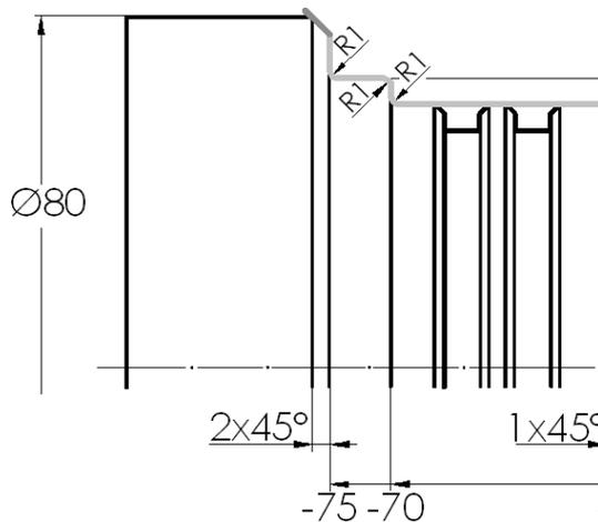
Chamfer and tangential leaving of the contour
