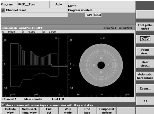
Simulation in the 2-side view which you can call via the softkey .
