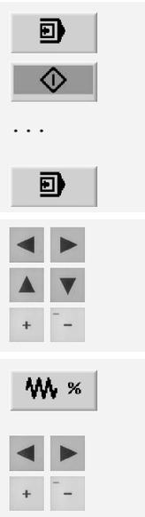
then use the softkey [Single Block] to switch to single block simulation. The simulation will stop after each block; to continue, press [NC Start].
