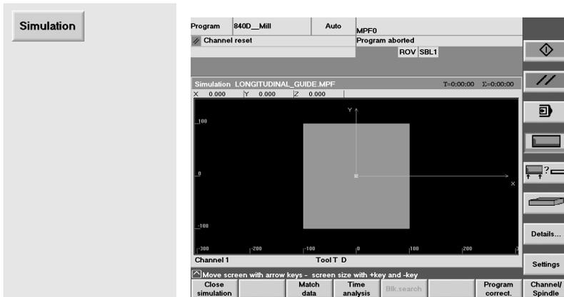
The simulation graphics is created and the workpiece is shown in top view (see softkey with the \*\*\*türkisfarbenenem\*\*\* margin).
