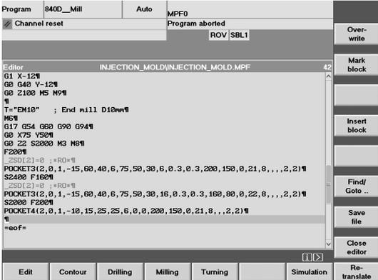
The cycle for the circular pocket has been accepted into the program. The cursor is now in the next (empty) line.
