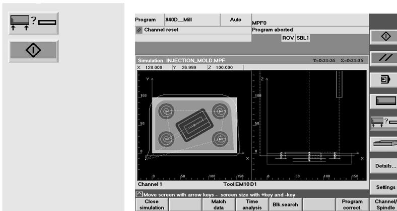
Simulation, here in the two-sides presentation (top view and front view)
