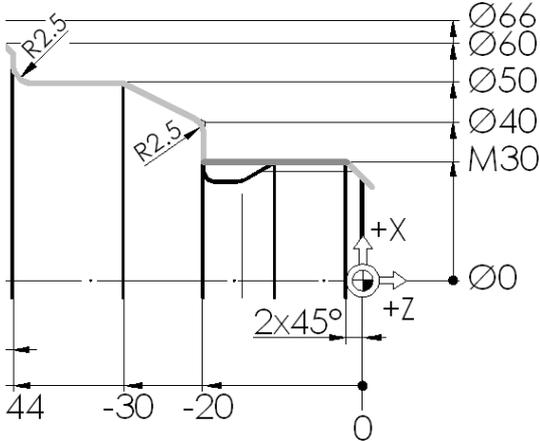
Horizontal skimming of the thread rated diameter.
