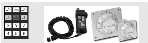
Traverse the tool carefully with the axis keys, a separate handheld unit or electronic handwheels until it comes into contact with the workpiece. (If necessary, you can then retract the tool vertically to the scratching direction and stop the spindle).
