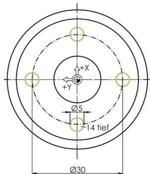
Instead of the cycle one could also have programmed the 4 drill positions via simple G0 blocks (cf. milling example "Longitudinal guide"). Now the compensation of both methods as they appear in the editor:
