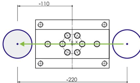
The cutter traverses at feedrate (feedrate 400 mm/min) along a straight line (G1) to the target point X-110 (absolute dimension referred to zero).
