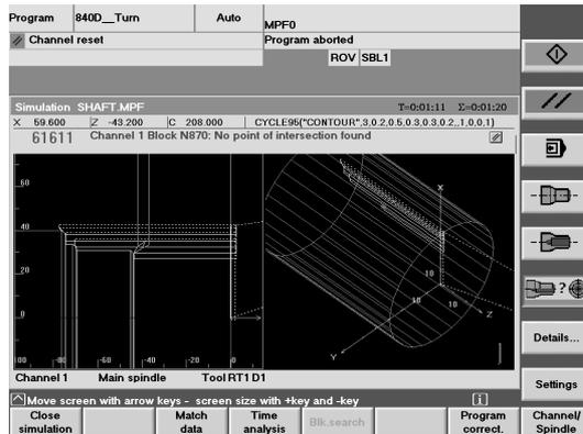
If you have detected an error in the simulation which is to be found, e.g. in the subroutine "CONTOUR" ...
