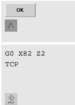
Press this softkey to accept the cycle into the program.
