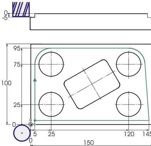
A point near the starting point A on the contour is approached as the starting position of the cutter in the XY plane.
