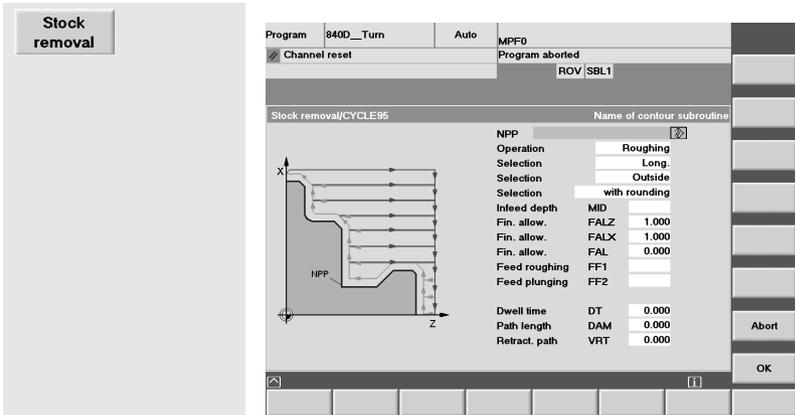
The dialog box for the cutting cycle CYCLE95 is opened by pressing the vertical softkey.
