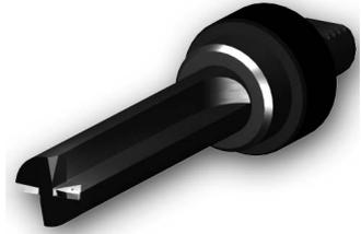
Drilling is carried out at constant speed (G97). Unlike turning, the spindle rotates clockwise (M3).
