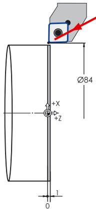
At first, the cutting tool is moved at rapid traverse (G0) from the tool change point to a position 2 mm above the workpiece.
