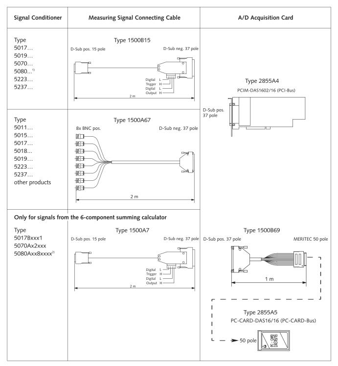
$^{\scriptscriptstyle 1)}$  Cable Type 1500B15 is used when output signals  $F_{x_{1}z_{2}},F_{x_{3}+4_{1}},F_{y_{1}+4_{1}},F_{y_{2}z_{3}},F_{z_{1}},F_{z_{2}},F_{z_{3}},F_{z_{4}}$  have to be acquired.
