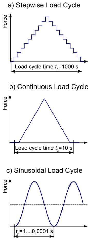
**Figure 1.1** Load-time dependence diagrams for stepwise, continuous and sinusoidal (dynamic) load cycles
