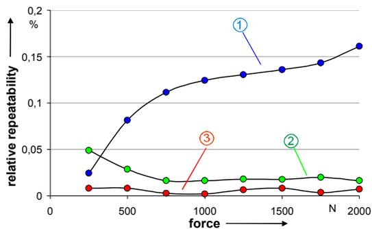
**Figure 4.2** Relative repeatability in the same mounting position at different time intervals  $\Delta t$  and under different drift conditions
