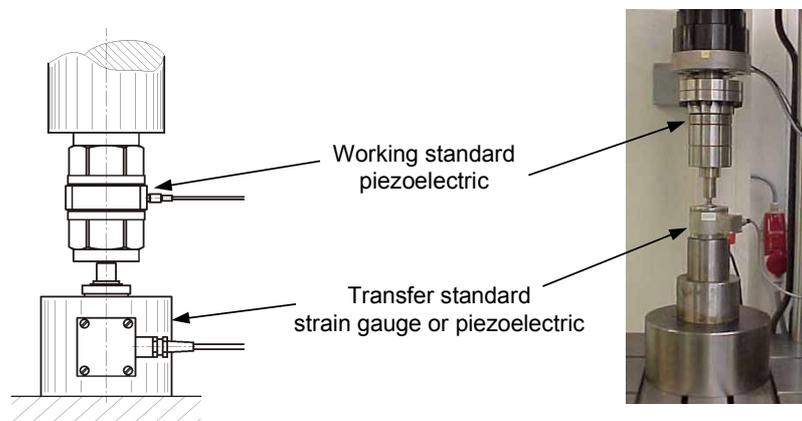
**Figure 3.2** Set up for working standard calibration
