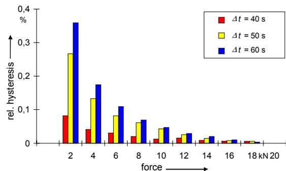
**Figure 4.4** Relative hysteresis (relative reversibility error) of a piezoelectric force transducer in the nominal load range of 20 kN
