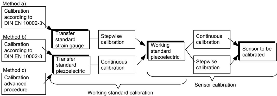
**Figure 3.1** Traceability and methods of piezoelectric working standard calibration
