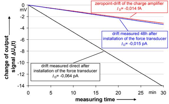
**Figure 4.1** Influence of electrostatic charges due to connectors and cables on the drift of piezoelectric force measuring devices
