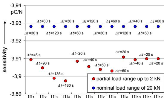
**Figure 4.5** Sensitivity of a piezoelectric force transducer in the partial load range up to 2 kN and in the nominal load range up to 20 kN at different time intervals  $\Delta t$
