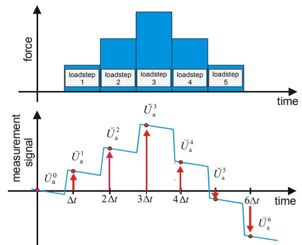
**Figure 2.1a** Load-time dependence diagram, 2.1b signal-time dependence diagram of a piezo-electric force measuring device according to DIN EN 10002-3
