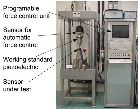
**Figure 3.3** Typical calibration facility comprising a servo-hydraulic press (200 kN), a piezoelectric working standard and a control unit
