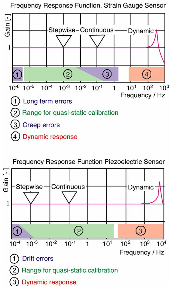
**Figure 1.2** Typical frequency response functions of a strain gauge sensor (top) and a piezoelectric sensor (bottom) compared to the load cycle frequencies of different load cycles
