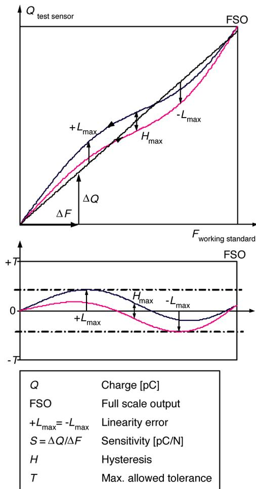
**Figure 3.4** Response curve of a continuous calibration with BSL (upper diagram). The signal of the sensor under test is plotted versus the signal of the working standard. The deviation between response curve and best straight line is plotted in the lower diagram.
