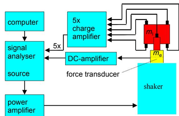
**Figure 2.2** Calibration facility for dynamic force measurement
