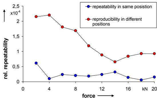
**Figure 4.3** Relative repeatability when the force transducer is loaded with a nominal force of 20 kN in the same and relative reproducibility in different mounting positions
